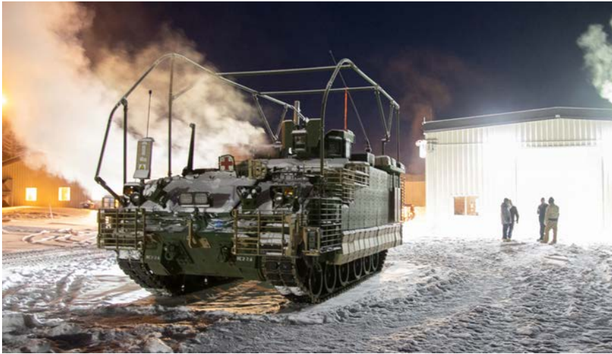
Figure 2. A multi-month evaluation at U.S. Army Cold Regions Test Center helped ensure the Army's latest armored personnel carrier works even in the world's coldest environments. The AMPV boasts the same powertrain and suspension system as the BFV and M109A7 self-propelled howitzer, which eases maintenance and logistics challenges for all three vehicles in the field. (U.S. Army photo by Sebastian Saarloos)
