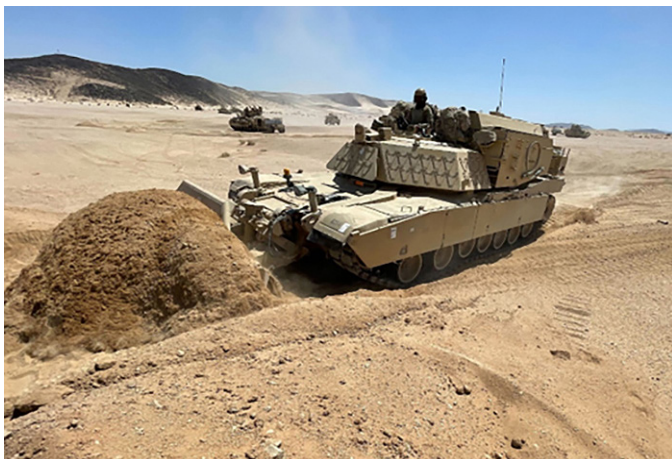
Figure 4. A 59 th CEC-A ABV proofs a lane during NTC 22-06 with 2 nd ABCT, 1 st Cavalry Division. (U.S. Army photo)
