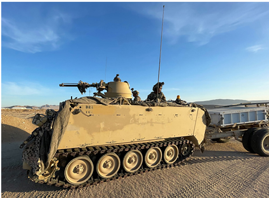
Figure 1. An 87 th Sapper M113 APC tows a MICLIC trailer at NTC, Fort Irwin, CA. (U.S. Army photo)
