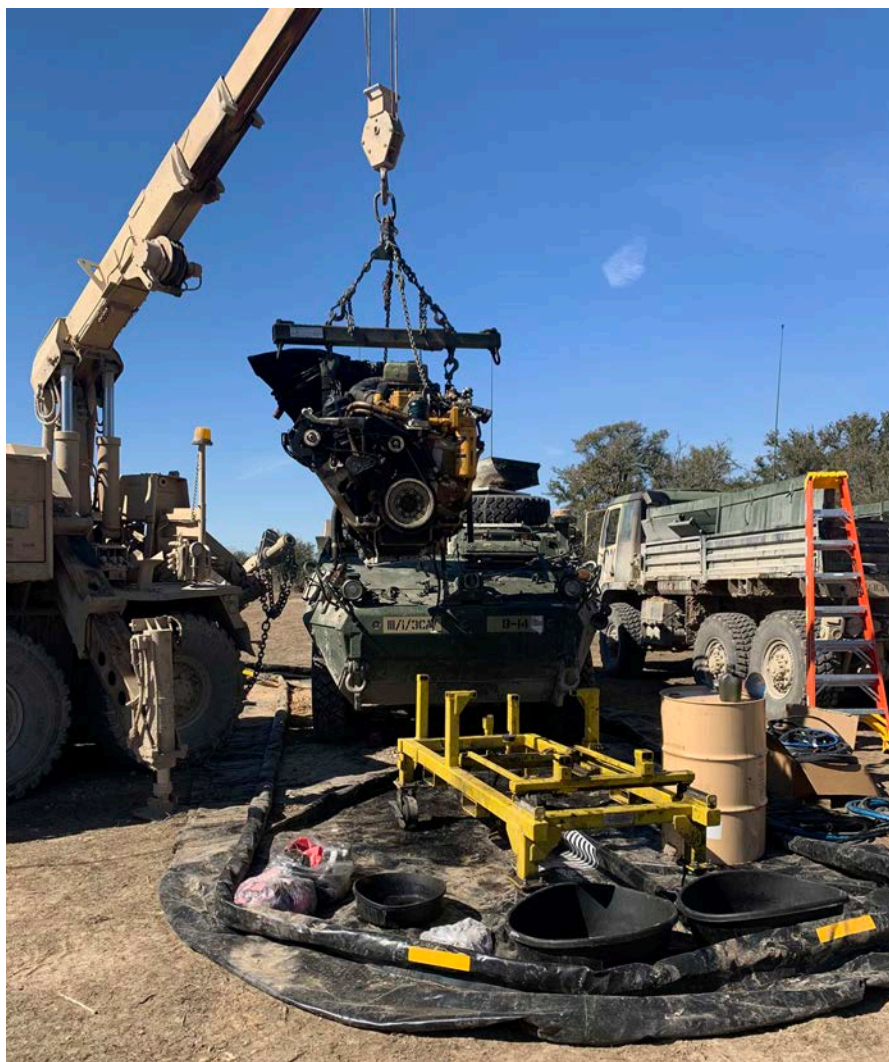
Figure 1. A pack change is made in the field during Operation Rifles Forge, a troop situational-training exercise/combined-arms live-fire exercise, at Fort Hood, TX. In February 2022. (U.S. Army photo by MAJ Patrick Kuiper)
